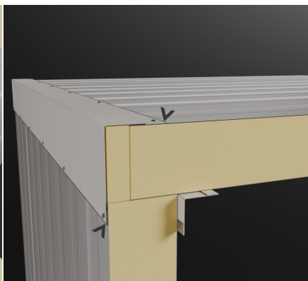
Steel plate cut at T-joint of partition wall .The T-joint has L-shaped edges sealed on both sides and secured with rivets.
